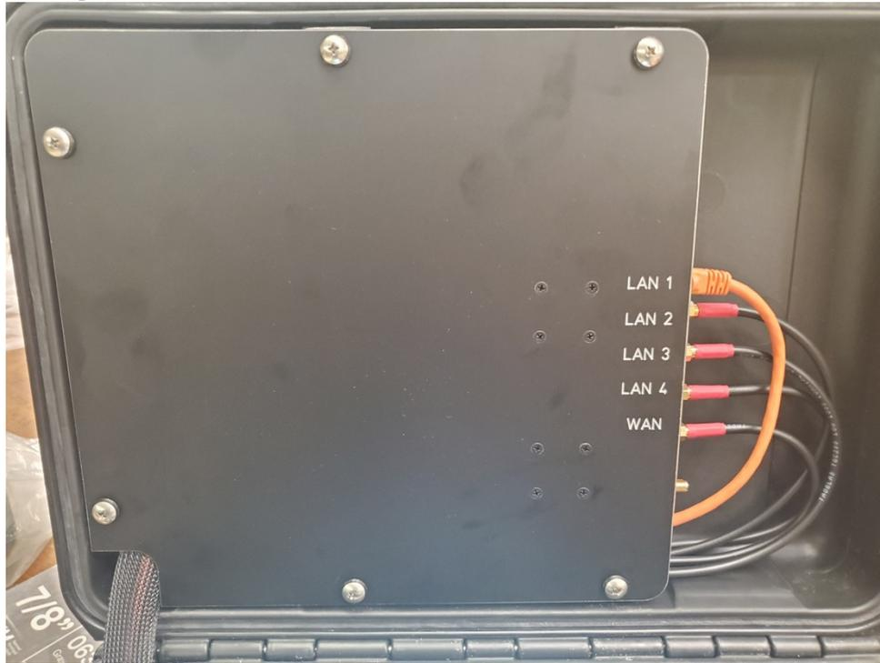
Then Remove the lid plate with the peplink attached, you can leave the antennae attached throughout the whole process. (Figure 6)
