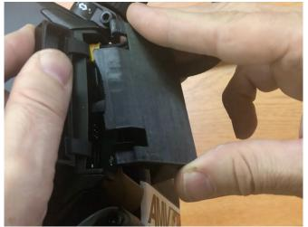
The final piece is adding the cable clip to support and hold the cable in place
