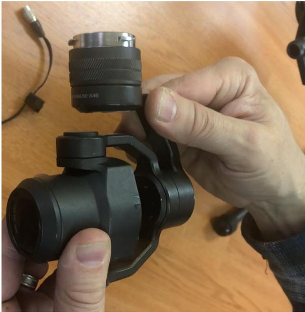
Slide the light “head” over the camera lens
