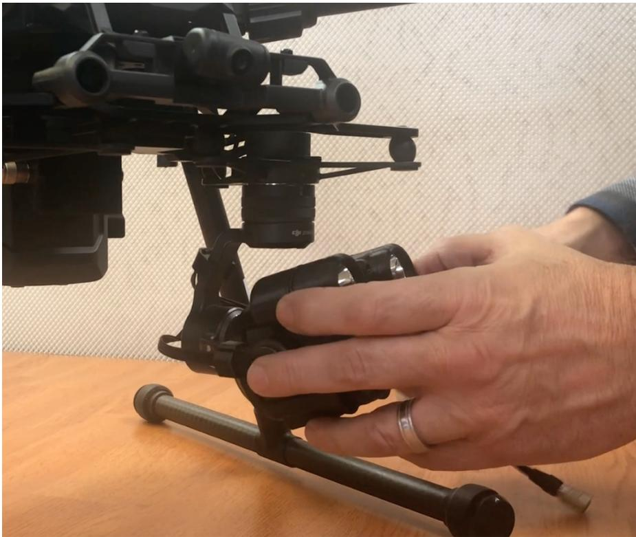
After connecting the camera, lay the loose remaining cable FLAT.
