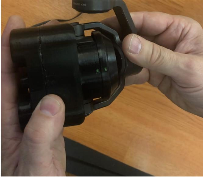
Connect the first clip on the attached cable to the right "rib" of the camera gimbal arm
