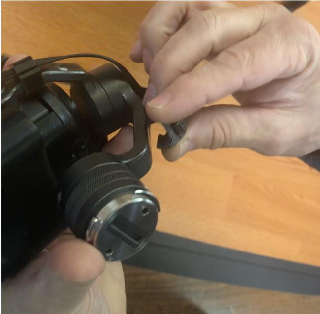
Connect the camera to gimbal 1 on the Matrice. In the image below you can see clips 1 and 2 in their final position.
