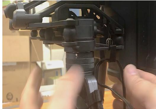
Finally, attach the connector to the Port side connector of the RemoraCBX
